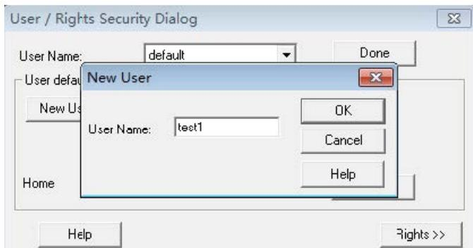
7. Enter the password of the user (for example, test1) created above in the **New Password** and **Verify Password** field respectively, and then click **OK**.
