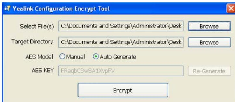
2. When you start the application tool, a file folder named “Encrypted” is created automatically in the directory where the application tool is located.
